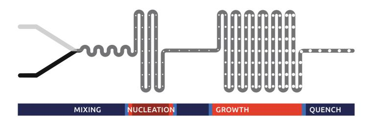
The growth of quantum dots is susceptible to minute changes in reaction conditions, the unique control that flow chemistry permits gave me precise and repeatable quantum dot growth.
