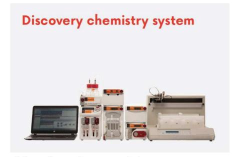
For limited quantities of starting material or expensive reagents, Asia Discovery Chemistry Systems offer setups capable of running flow experiments using very small amounts of reagents.
