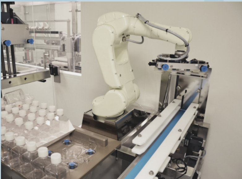
The robotic arm plays a crucial role in our new automatic filling machine.
