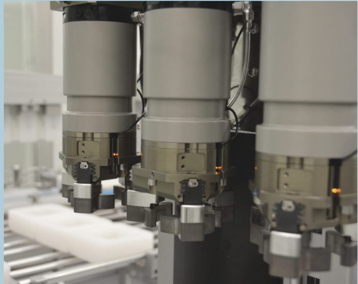
The motors and moving parts of the automatic filling machine are oil free.
