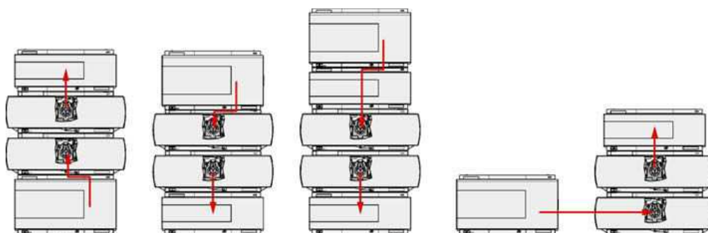
Figure 5 Different system set up possibilities with 2 column compartments. Only the autosampler (if necessary with thermostat) and a DAD as detector are shown. In the dual-stack setup note that the autosampler and the lower TCC are at the same level, also a distance of both stacks of 8 cm should be met.
