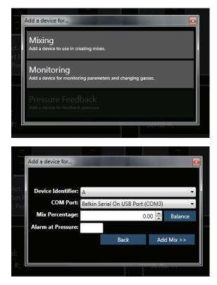
Select **Mixing** to add a device that will be used for gas mixing. Enter the following information:
