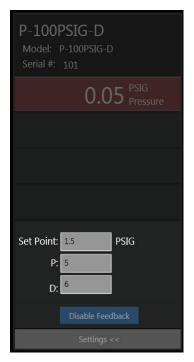
Flow Vision MX uses a modified PID control algorithm to maintain pressure at a set-point.
