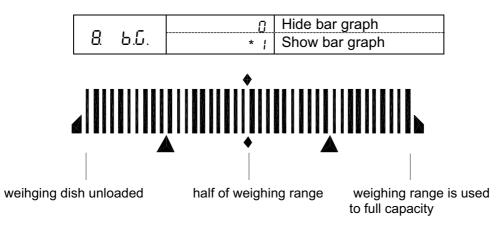
The weighing range of the balance is divided into 40 graphic cuboids. Zero (0) will appear on the graphic display if there is no weighing value on the balance. 20 graphic cuboids are displayed if the balance is loaded up to one half of its weighing range.
