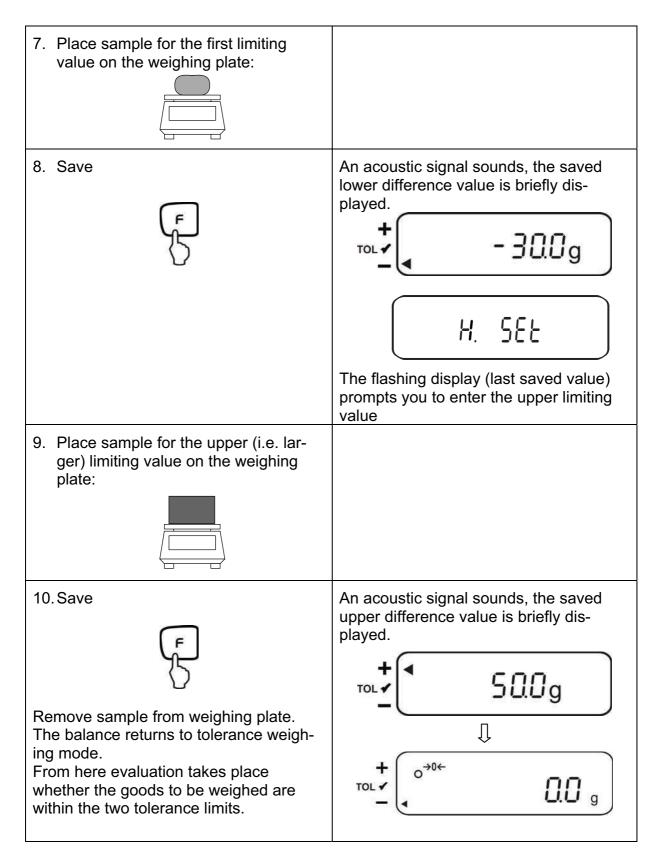
\* If you want to set for your tolerance weighing only one limit point (parameter selection [23. P. 1]), the input herewith is finished.
