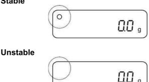
If the display shows the stability display **[o]** the balance is in a stable status. The **[o]** indication disappears if the condition is unstable.
