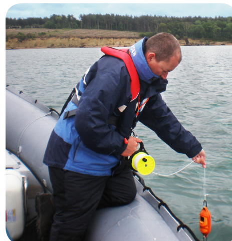
The CastAway incorporates the most modern technology available yet is simple to use. It is designed for profiling down to 100 m and is easy to deploy.
