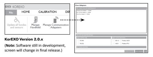
**USB passthrough drivers** will automatically be installed along with KorEXO 2.0 software, they are also available separately from the **EXOwater.com** website. Install these drivers on your PC to communicate with a signal output adapter (SOA) through any version of Desktop KorEXO:
