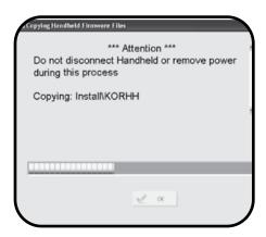
**NOTE:** Firmware updates require all instrumentation (Handheld, sonde, sensors, and desktop software) be updated to function properly.
