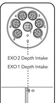
The sonde should be installed with at least 1 cm of water above the intake ports. If a conductivity sensor is installed, the depth will be compensated automatically for changes in the density of water as temperature and salinity change.
