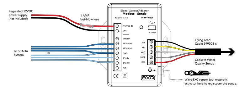
**Note:** The orange wire on the flying lead cable to the sonde will not be used. It can be taped back during installation.
