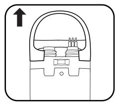
Once screws are removed, lift the bail off the sonde.
