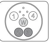
EXO3 Optimal Wiped C/T positions: 2 or 3
