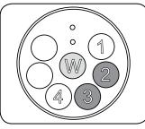
EXO2 Optimal Wiped C/T positions: 2 or 3
