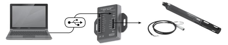
**Note:** USB utilizes Communication Device Class (CDC) and installs as comport on PC: "YSI SOA/DCP Gen2". The USB connection may also be used to update firmware on the adapter using KorEXO software.
