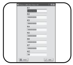
In the Advanced menu, click the Edit button and enter the unique membrane cap coefficients found on the instruction sheet shipped with the DO sensor cap.
