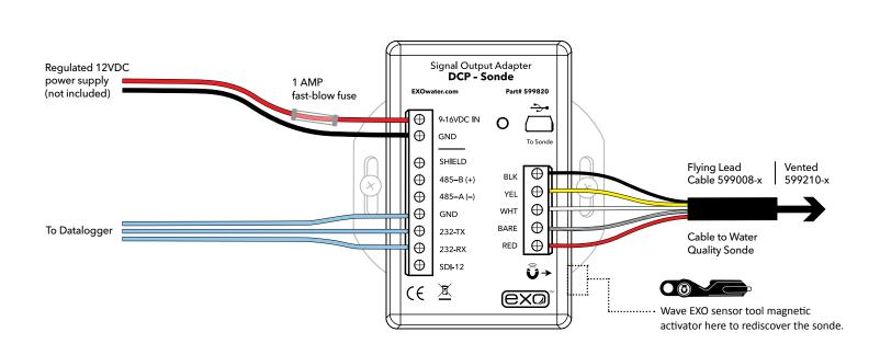
When connecting new sondes to the DCP adapter, it may be necessary to redetect the sonde. This can be done by power cycling the adapter or by using the magnetic read switch at the lower right hand side of the enclosure. Waving the magnet in the EXO sensor tool over the area referenced by the square above, will force a network redetect where all new sensors and configurations will be discovered.
