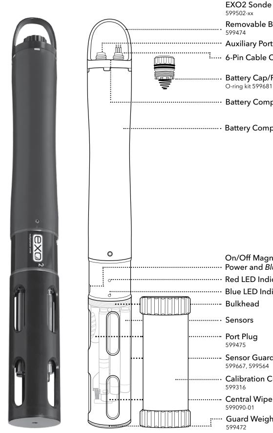
Removable Bail ···· Auxiliary Port ..... 6-Pin Cable Connector ...... Battery Cap/Pressure Relief Valve
