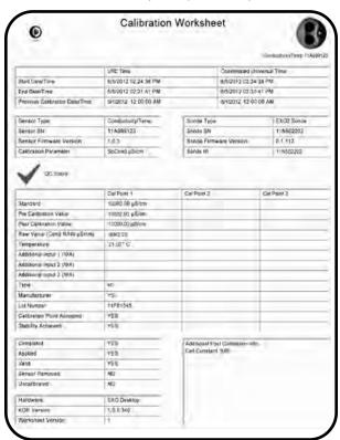
1-point calibration of percent saturation on EXO optical dissolved oxygen probe
