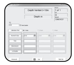
In the desktop KorEXO Calibrate menu, select Port D-Depth, then select Depth m from the second menu. In the Device Calibration menu, you should see Depth Vented 0-10m as the device name. (In the handheld KorEXO Calibrate menu, select Port D Dep V 0-10m, then select Depth m from the next menu.)
