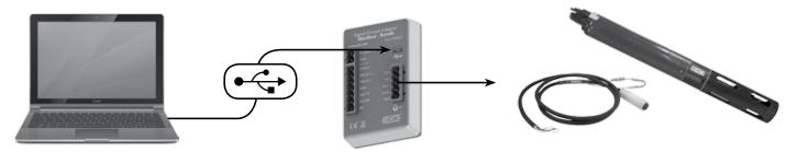
**Note:** USB utilizes Communication Device Class (CDC) and installs as com port on PC: "YSI SOA/DCP Gen2". The USB connection may also be used to update firmware on the adapter using KorEXO software.
