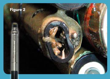
**Standard (C/T) Sensor** impacted by the accumulation of biofouling. (Red data in the plots.)
