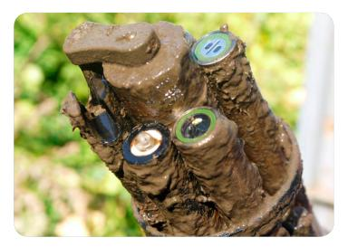
Combat particulates, algae, barnacles, and other types of foulting in long-term monitoring with EXO's Wiped (C/T) Smart Sensor.
