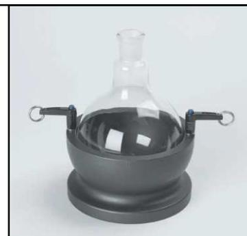
Handles should always be removed from block when heating. If handles are left in block whilst heating they will become hot.
