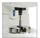
Thermal Barrier reduces the effects of heat transfer to the environment. Two part chamber provides thermal isolation of the measurement zone.
