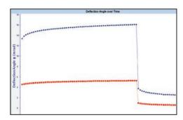
**Recovery:** Elastic property of material is characterized by spindle relaxation (backward rotation) after constant stress is removed.
