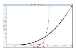
**Yield Stress Determination:** shear stress ramp from 0 to 800 Pa over 2 minutes shows yield stress values of 200 and 400 Pa for two materials.
