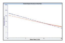
**Viscosity Flow Curve:** controlled shear stress ramp produces viscosity vs. shear rate graph for two pseudoplastic materials.
