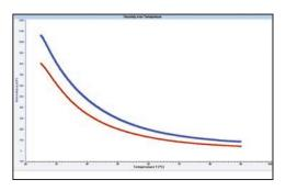
**Temperature Profile:** Viscosity is measured at constant shear rate of 250 1/s while temperature increases from 25°C to 90°C using RST Cone Plate Rheometer.
