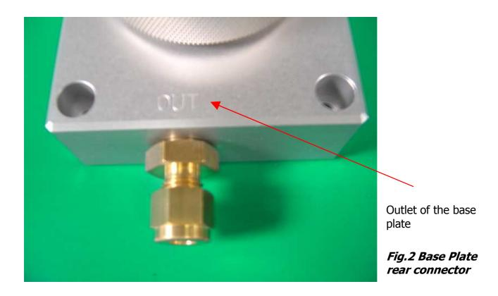
**3.** Insert the Particle filter with the Port connector side (see fig. 1) into the outlet side of the base plate (see fig. 2) as shown in fig.3 A and fig.3 B.
