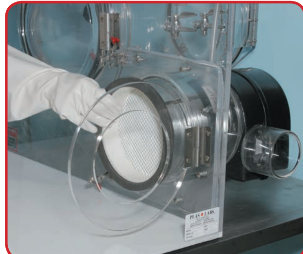
800-HEPA/S with filter access door open. Internal view (when changing filters)
