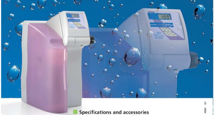
TKA MicroMed Permeate performance at 15 °C: 6 l/h Flow rate: 1.0 l/min Operating pressure in bar, min/max: 1 – 6 bar Conductivity: 0.1 - 1.0 µS/cm Resistance at 25 °C: 10 – 1 MΩ×cm Percentage of germs, bacteria, particles retained by the membrane: 99 % Supply voltage: Automatic voltage regulation to 24 V Power consumption: 0.06 kW Connector size: R 3/4" 305 x 400 x 545 Dimensions, W x D x H in mm:
