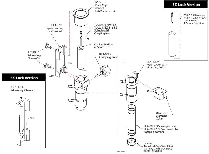
Figure 1: Enhanced UL Adapter Assembly
