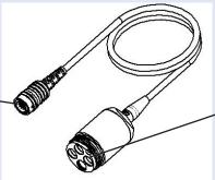
Four ports for user-replaceable sensors. Ports accept a temperature/ conductivity combo sensor, DO sensor, and any combination of two ISE sensors among pH, ORP, ammonium, chloride, or nitrate. If a port isn't used simply put a port plug in it's place.
