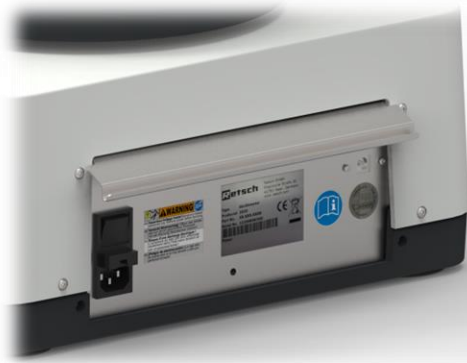
Fig. 15: AS 200 digit cA with splash protection
