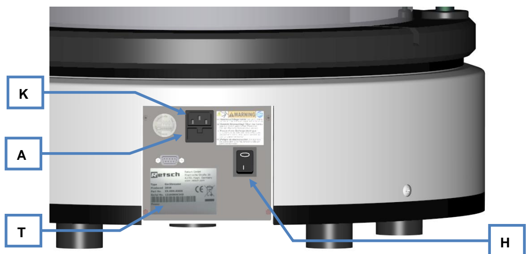
Fig. 17: Replacing the fuses
