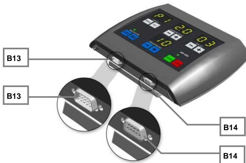
Fig. 8: Graphic Representation of the Control Panel Connection
