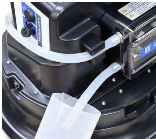
Calibration with large graduated cylinder
