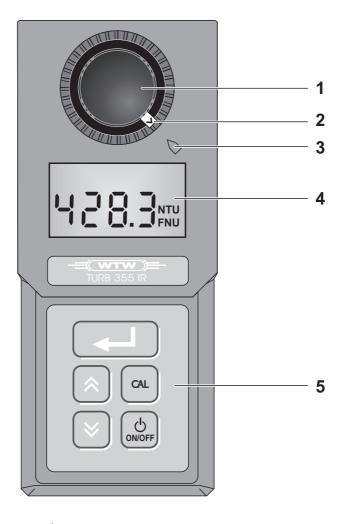
1 Cuvette in the cuvette shaft
