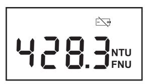
In this case, change the batteries immediately. The instrument might no longer measure with the specified accuracy. If the batteries are too weak to measure, the turbidimeter switches itself off. It can only be switched on again when the batteries have been replaced.
