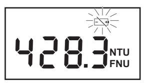
The batteries are nearly empty and should soon be exchanged. The instrument still measures with the specified accuracy.
