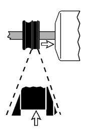
The side with the sharp-edged notch must show to the armouring head!
