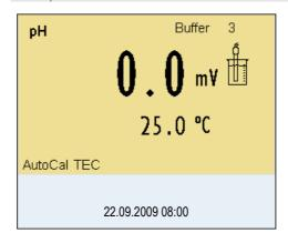
Finish the calibration procedure as a two-point calibration with <M>.
