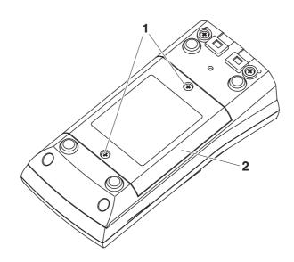
3 Place four rechargeable batteries (type Mignon AA) in the battery compartment.
