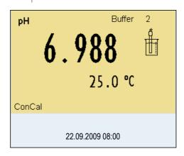
8 If necessary, finish the calibration procedure as a single-point calibration with <M>.
