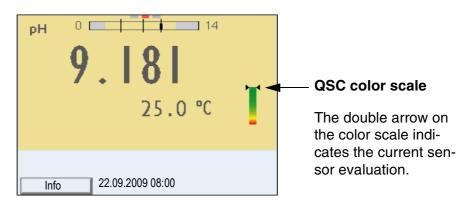
The sensor evaluation is documented as a percentage (1 - 100) both in the calibration record and for individual measurement datasets.
