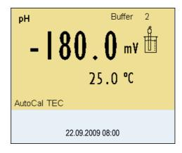
If necessary, finish the calibration procedure as a single-point calibration with <M>.
