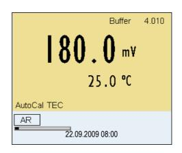
15 Use <M> to finish the calibration. The calibration record is displayed. or Switch to calibration with the next buffer with <MENU/ ENTER>.
