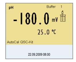
Calibration with the buffers of the QSC-Kit is done like a normal three-point calibration.
