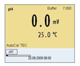
10 Wait for the measurement with stability control to be completed or terminate the stability control and take over the calibration value with **<MENU/ENTER>**. The calibration display for the next buffer appears.
