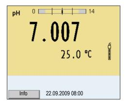
1 In the measured value display: Display the sensor data (sensor name, series number) with [*Info*].
