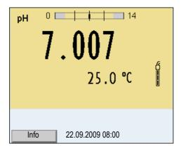
Switching off Press the <On/Off> key.
