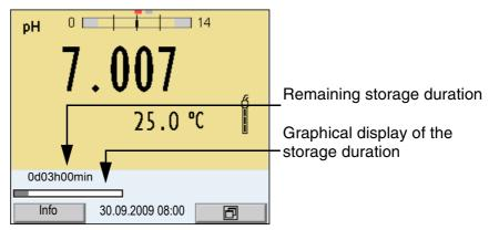
The active automatic storage function can be recognized by the progress bar in the status line. The progress bar indicates the remaining storage duration.
