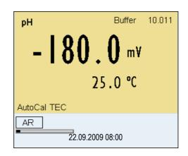
5 Wait for the end of the measurement with stability control or accept the calibration value with **<MENU/ENTER>**. The calibration display for the next buffer appears.
