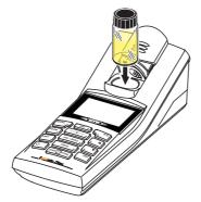
3 For turbidity measurement: Align the cell (see section 4.7.2).
