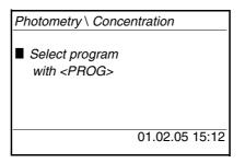
With <M> (long pressure) change the measuring mode. With <M> (short pressure) toggle between the different measured parameters in the selected measuring mode.
