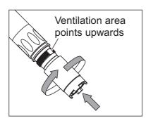
Hold the sensor inclined and screw on the membrane cap fingertight using a paper towel. Excess electrolyte solution is forced out of the ventilation area.
