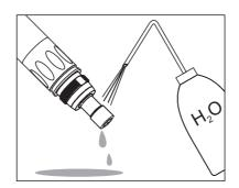
Rinse the sensor head with deionized water.
