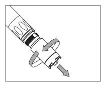
Unscrew the membrane cap. Caution: Electrolyte solution! For disposal of the membrane cap and electrolyte solution, see section 5.7.
