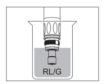
Immerse the sensor head including the counter electrode in RL/G cleaning solution.
