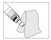
Wipe the counter electrode with a lint-free paper towel and carefully remove any loose white deposits.
