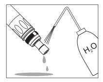
Rinse the sensor head with deionized water.
