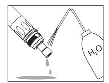
Thoroughly rinse the sensor head with deionized water.
