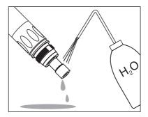
Rinse the sensor head with deionized water.
