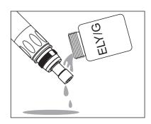
Rinse the sensor head with electrolyte solution.
