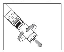
Unscrew the membrane cap. <u>Caution:</u> Electrolyte solution! For disposal of the membrane cap and electrolyte solution, see section 5.7.
