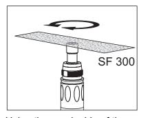
Using the rough side of the wet SF 300 polishing strip, polish off any contamination from the gold working electrode using light pressure.
