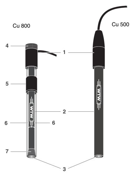
Connection head with connection cable
